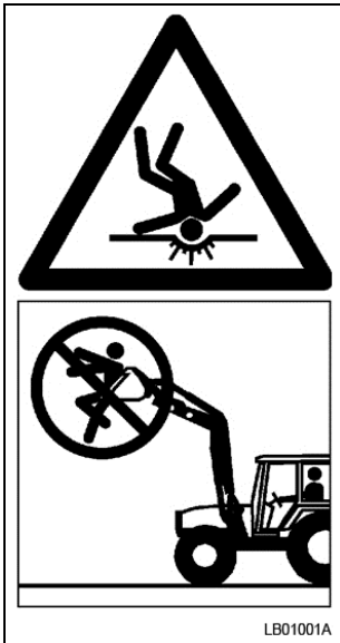
Fig. 3: Person at risk if lifted by the frontloader.
