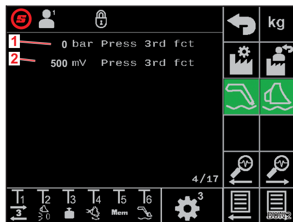
Fig. 40 Pressure sensor in 3rd control circuit
